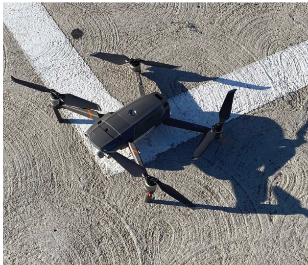
Figure 3. Tactical drone (weight: 2 pounds; speed 45 mph; flight time: 28 minutes; dimensions: 322mm x 242mm x 84mm)
