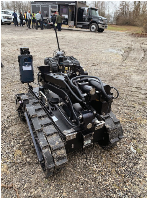
BearCat EOD with BWC attached with bike handlebar phone mount.
