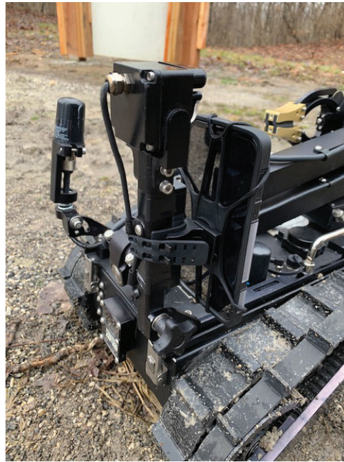
BearCat EOD with BWC attached with bike handlebar phone mount.
