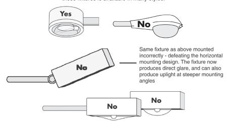
Known as just "Cutoff". Center "drop" or "sag" lens with or without exposed bulb, produces direct glare.
